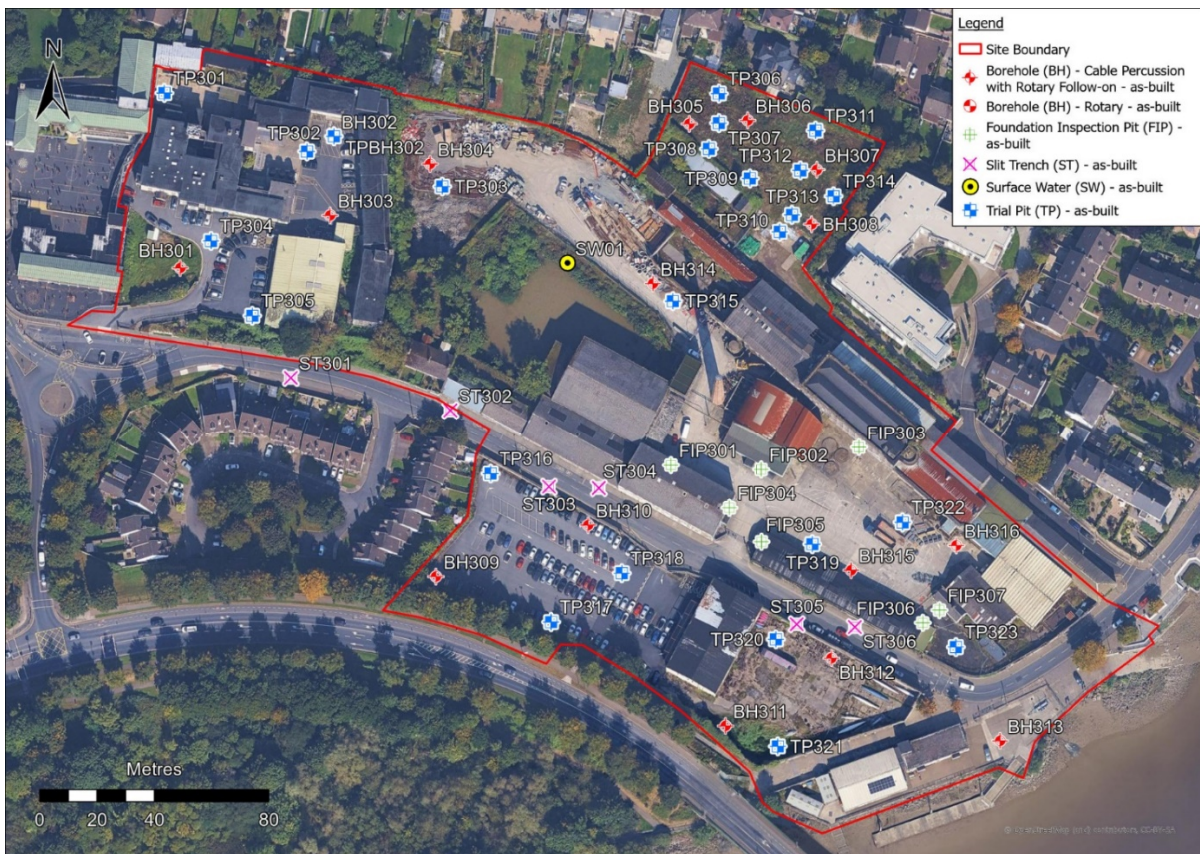
Figure 3: As-built exploratory locations undertaken during the PGL 2025 GI.
